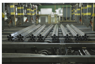
Manufacturing torches using recycled aluminum
